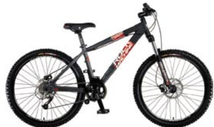
Stampede70 FRAME Block Design Custom 7005 DB FORK Marzocchi Dirt Jumper 3, 100mm DERAILLEUR Shimano LX SHIFTERS Shimano Deore BRAKES Hayes HFX 9 V7 w/BFL Disc CRANKSET Truvativ Hussefelt 1.0 BG, 38T + boxguide FREEWHEEL Shimano HG50, 11-32T WHEELSET Rock Machine + chain tensioner, Mach1 Freeride Disc, Kenda Kinetics, 2.35 SIZES 14", 15.5" € 1099,-
