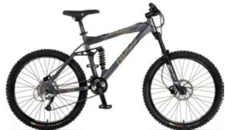
Adrenaline5000 FRAME Alpine Custom 7005 DB REAR SHOCK Manitou Metel RP, 150mm FORK Marzocchi Z1 Sport RV, 150mm DERAILLEURS Shimano LX / LX SHIFTERS Shimano Deore BRAKES Hayes HFX 9 V7 w/BFL Disc CRANKSET Truvativ Hussefelt 2.0 RG, 22/32T FREEWHEEL Shimano HG50, 11-32T WHEELSET Rock Machine, Mach1 Freeride Disc, WTb Timber Wolf Steel DNA, 2.3 SIZES 17", 18" € 1299,-
